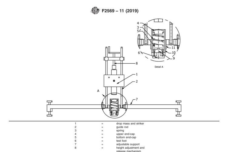
FIG. 1 Force Reduction Test Apparatus
